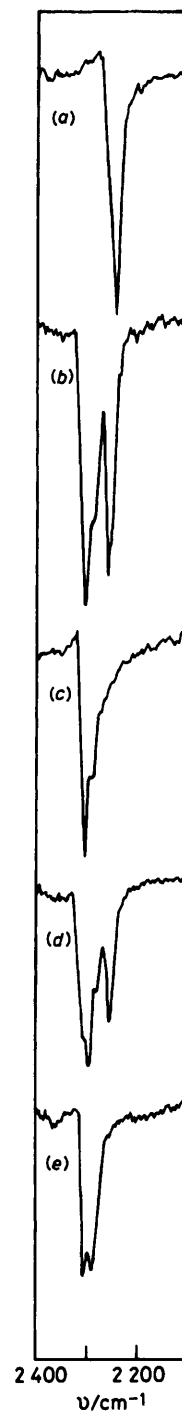
Figure 2. CN Stretching absorptions in (a) P(CH_2CH_2CN)_3O ; (b) ZnCl_2 \cdot P(CH_2CH_2CN)_3O ; (c) 2CoCl_2 \cdot P(CH_2CH_2CN)_3O \cdot 3H_2O ; (d) cobalt complex in (c) after prolonged heating; and (e) 3NiCl_2 \cdot 2P(CH_2CH_2CN)_3O \cdot xH_2O
